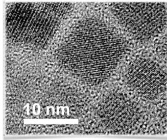
PeQD is an advanced material that is made by microfabricating perovskite semiconductors. Its shape is a very small particle equipped with a ligand, about 10,000 times thinner than a human hair. It is attracting attention as a next-generation light-emitting material with high PLQY, high color purity, and high color adjustability.
