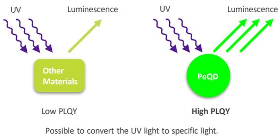
Light-emitting materials such as PeQD absorb light unique to each material, convert the wavelength, and emit light. In particular, PeQD has extremely high light conversion efficiency and can achieve a luminescence quantum yield (PLQY) of 100%, which is an indicator of conversion efficiency.
