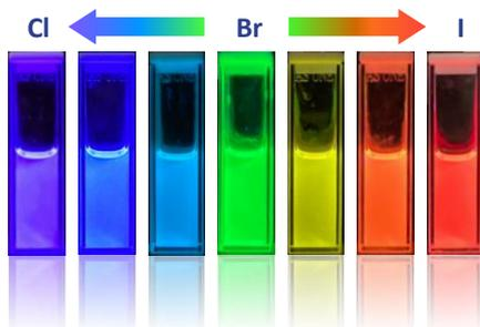
By controlling the halogen ratio and particle size, PeQD can control the emission color from purple to red. By combining these technologies and creating an optimal synthesis recipe, it is possible to easily tune all colors of visible light.
