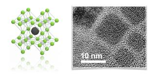
PeQD is an advanced material that is made by microfabricating perovskite semiconductors. Its shape is a very small particle equipped with a ligand, about 10,000 times thinner than a human hair. It is attracting attention as a next-generation light-emitting material with high PLQY, high color purity, and high color adjustability.
