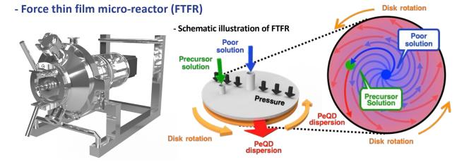
Our groups developed a scale-up preparation method of PeQD by FTFR, which is the continuous flow process. By mixing the precursor solution and poor solvent in the two disks, it is possible to mix two solvents uniformly, resulting in obtaining PeQD dispersion with high optical properties continuously. In addition, PeQD with almost the same properties can be synthesized based on LARP recipes.
