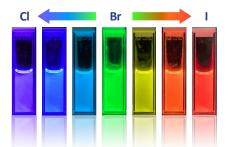
Light-emitting materials such as PeQD absorb light unique to each material, convert the wavelength, and emit light. In particular, PeQD has extremely high light conversion efficiency and can achieve a luminescence quantum yield (PLQY) of 100%, which is an indicator of conversion efficiency.
