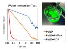
Significantly reduced PL degradation by the PeQD-polymer composited materials.
