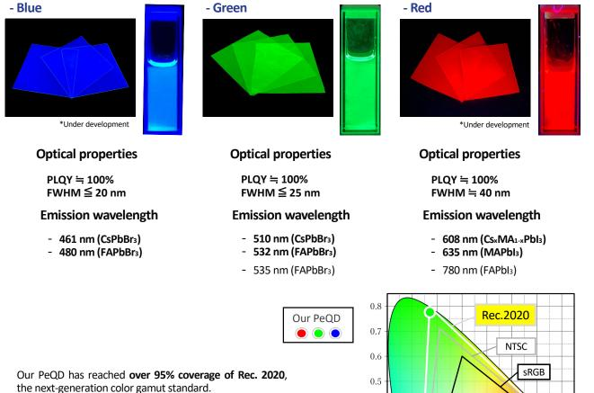
We aim to develop LEDs based on PeQD materials and implement them in displays.
