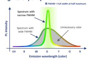
Light-emitting materials such as PeQD absorb light unique to each material, convert the wavelength, and emit light. In particular, PeQD has extremely high light conversion efficiency and can achieve a luminescence quantum yield (PLQY) of 100%, which is an indicator of conversion efficiency.
